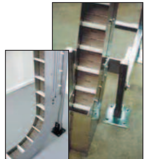
Defense: 90-degree vertical bend with a cleated 450 series segmented belt
