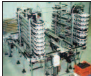
Electronics: Alpine vertical conveyors with custom part carriers
