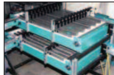
Electrical: High density, stacked serpentine part accumulators
