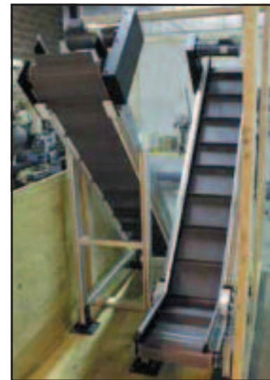
Appliance: Segmented, cleated belt incline scrap conveyors
