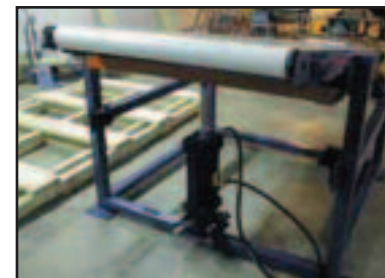
Building Materials: Belt conveyor equipped with an automatic incline actuator
